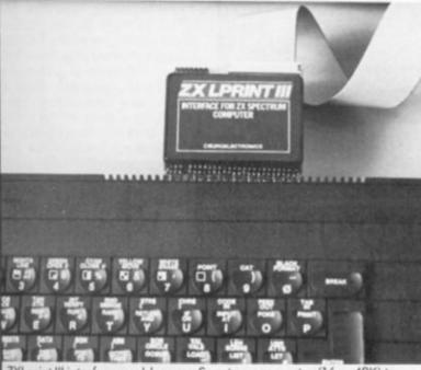
ZXLprint III interface enables your Spectrum computer (16 or 48K) to print on almost any dot matrix or daisy wheel printer with RS232 or Centronics input. Just plug in ZXLprint III and LPRINT and LLIST commands will work. COPY works without any software on Epson, Star Delta, Brother HR5 & 1009, Gemini, Walters WM80, Mannesman MT80, Kaga Taxan, Cannon, Shinwa, Seikasha 100, 250 & 500. Plus Seikasha GP700 in FULL COLOUR. Also available is optional COPY in 4 colours on CGP115, MCP40 & 80 and SCP80.
